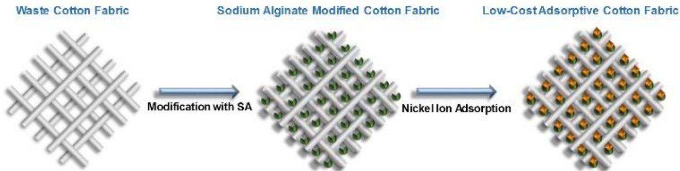
Scheme 1. Schematic of the experimental strategy, including the fabrication of SA-modified waste cotton fabric and the adsorption of nickel ions using the SA-modified waste cotton fabric
